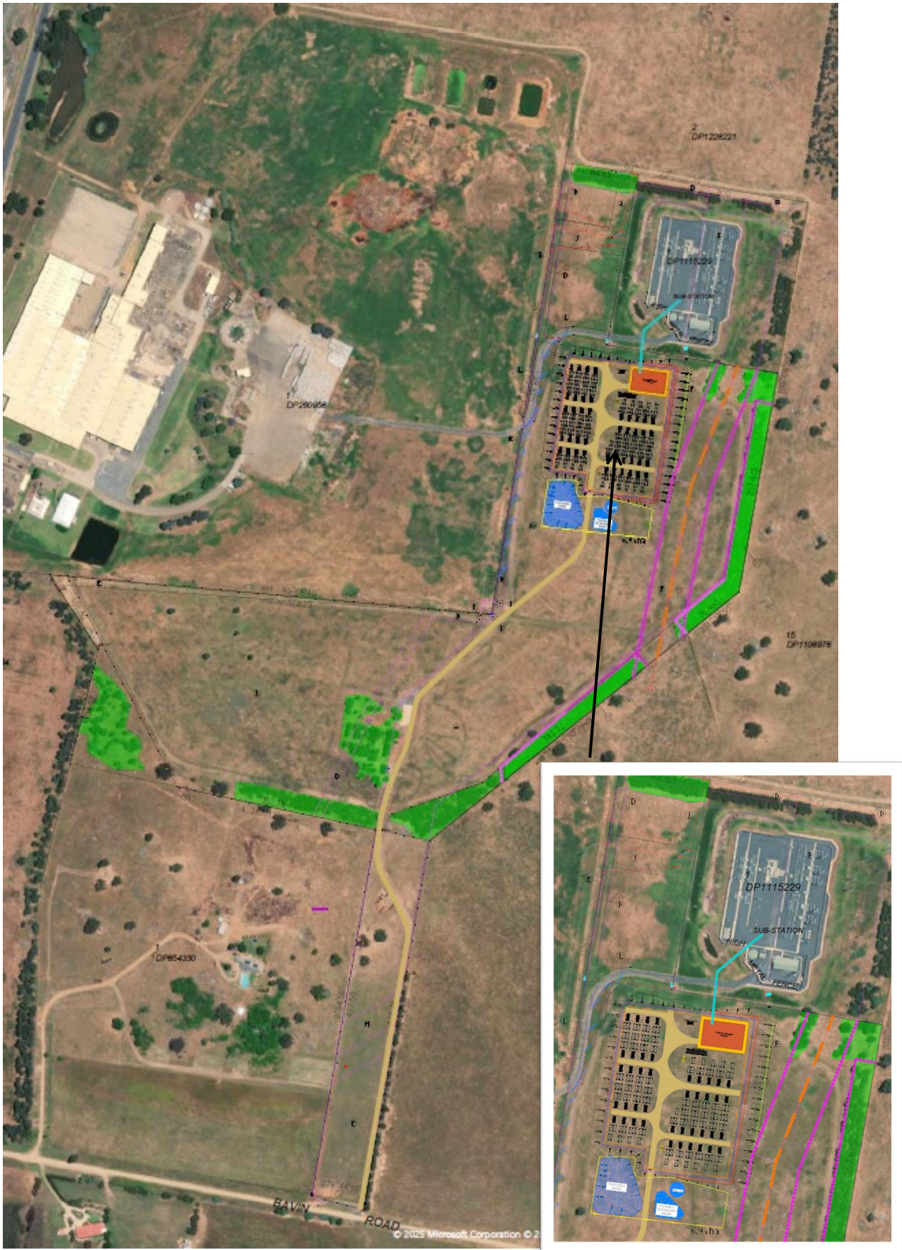
Figure 1-1 Preliminary design of the proposed development with existing transmission line easements shown as purple dashed line and native plantings shown in green. Proposed access road in light brown.
